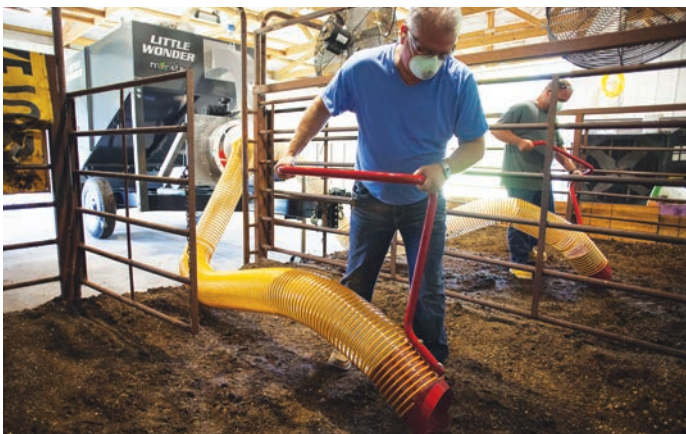
Dual 15' Hoses feature anti-friction, anti-clog smooth-bore interiors, for uninterrupted work
