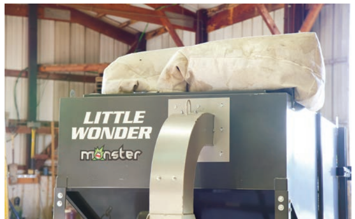
Top-vented with felt bags for increased filtration
