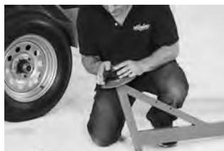
3. **⚠ WARNING:** The Bearing is not secured to the Boom base. Keep your hand under the Bearing when lifting or stalling the Boom to the Discharge Stack.
