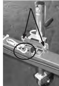
3. Install draw bar into trailer frame with two 5/8" x 1/2" bolts and two 5/8" lock nuts (Tow Behind Only).
