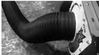
3. Loop one ratchet strap around the intake hose so that the ratchet hardware is on the top side of the intake flange. Insert the end of the strap into the ratchet hardware.
