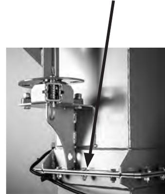
7. Install discharge hose 12" heavy duty clamp with 6-1/2" X 1" bolts.
