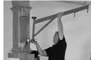
6. Swing the Boom Arm into the Boom Lock Pin
