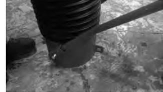
2. Loop the remaining ratchet strap around the intake hose so that the ratchet hardware is on the top side of the nozzle between the handle and ratchet the strap tightly around the nozzle.
