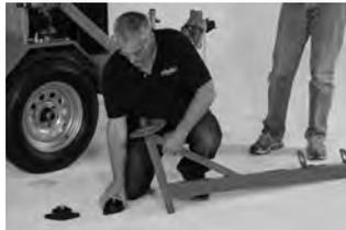
2. Place a Boom Arm Support Bearing over top of Fiber Washer over **BOTTOM** of Boom.
