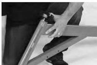
5. Supporting the base (bottom) Boom Support Bearing when lifting the Boom Assembly, slide the Boom on to Discharge Stack Support Brackets
