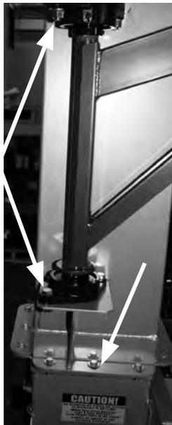
6. Install the debris elbow to the stack using 12-3/8" X 1-1/4" bolts, 24-3/8" flat washers, 12-3/8" lock washers and 12-3/8" nuts.
