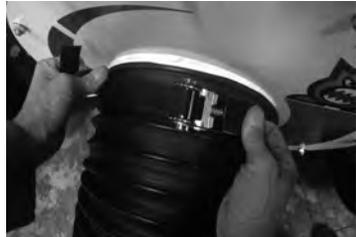
4. Use the ratchet to tighten the hose to the flange. Hold the strap with the other hand.
